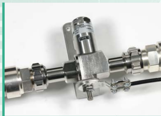
Befestigung des DEHNgate Art.-Nr. 929 146 mittels Erdungsschraube am Befestigungswinkel Art.-Nr. 106 310 und am Erdungskabel Art.-Nr. 416 411 Fixing of DEHNgate Part No. 929 146 with earthing screw at the angled fixing plate Part No. 106 310 and at the earthing conductor Part No. 416 411
