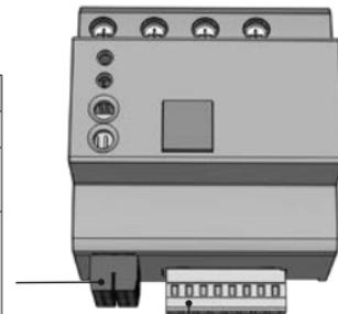
A slotted screwdriver ( $\leq 2.5 \text{ mm}$ ) is required to unlock the push-in connectors
