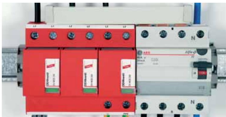
Fig. 8.1.6.11 V-shape series connection of the DEHNventil M TNC combined lightning current and surge protective device by means of a busbar
