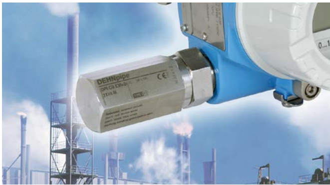
Surge arrester for outdoor use to be screwed onto two-wire field devices. Stainless steel, installation with cable gland up to IP 67.
