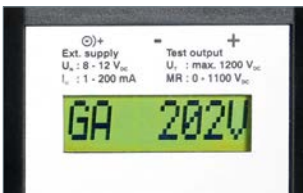
Indication of the measured spark-over voltage.
