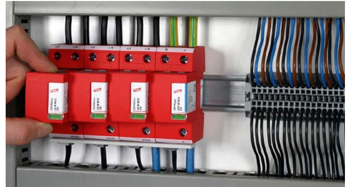
For protecting low-voltage consumer installations against surges and even direct lightning strikes. For installation in conformity with the lightning protection zone concept at the boundaries from 0 A -1 (3+1 configuration).
