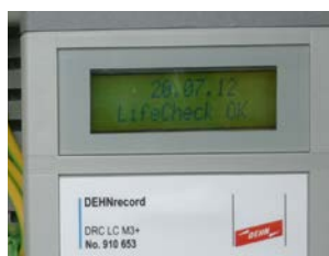
Interval testing with DRC LC M3+.
