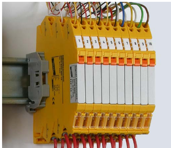
Application example: DEHNconnect for protecting the I/O of PLC interfaces.
