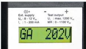
Indication of the measured sparkover voltage.
