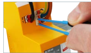
Integrated test ports for testing the signal circuit by means of test pins.
