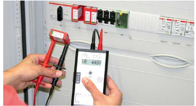
For testing the sparkover voltage of surge arresters. The specimen is connected via the test leads supplied or special test adapters.
