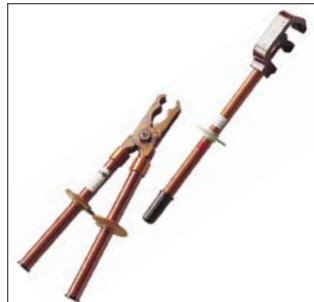
Old fuse tongs – hazard of electric shock
